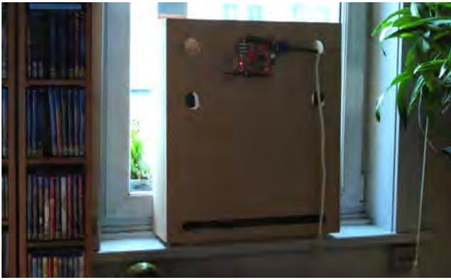
**Figure 1. Display casing with attached mini-computer, cable to power supply and ventilation holes.**
